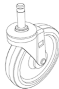
Option 'A' Castor 4 Inch Stem Fitting Castor Part No 628425
